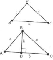
Construct an altitude, h, from one of the angles to the side opposite the angle. The two triangles formed,  $\triangle$ ABD and  $\triangle$ BCD, are right triangles.
